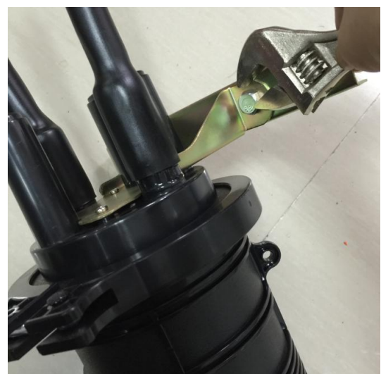
10. Fix on the hanging hook by wrench
