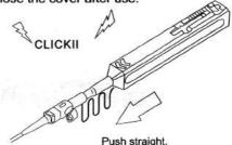
Be careful not to slant MU/LC connector while inserting into the Guide cap.
