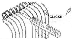
Be careful not to slant the CLE-PEN Cleaner MU/LC while inserting into the adapter.
