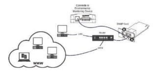
When the network interface cable is connected, the SNMP Card will attempt to obtain an IP address via DHCP. See "Configuration methods" on page 6.
